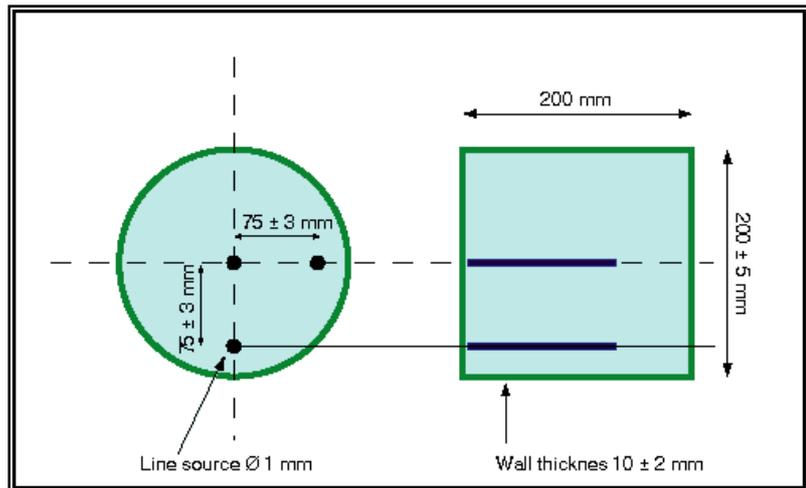
containing three axial line sources with diameter of 1 mm, figure 11. X.
